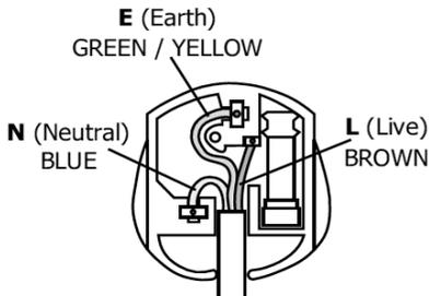
The wires in the mains lead are coloured in accordance with the following code:
