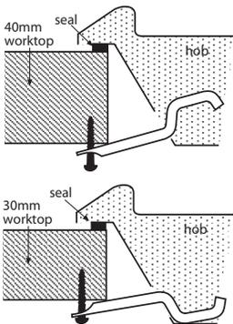
The screws should be tightened just sufficiently to secure the hob and pull the top pressing flush with the worktop. If the base of the hob is accessible after installation then a partition must
